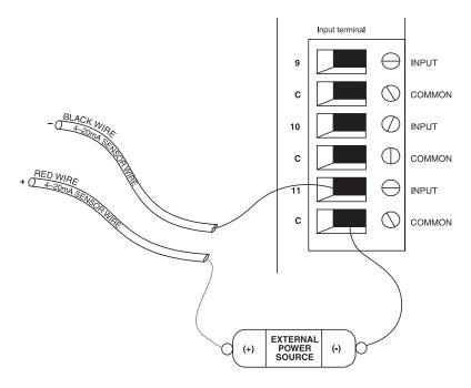
Figure 7: 4–20mA sensor using external power source
