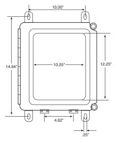
Figure 1: Mounting dimensions
