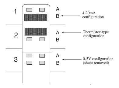
Figure 4: shunt configurations
