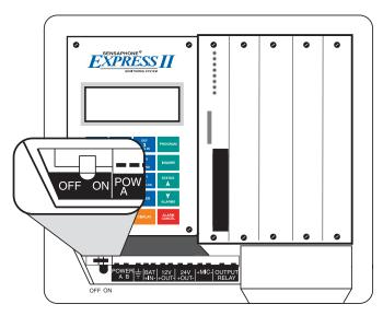
Figure 3: On/Off Switch Location
