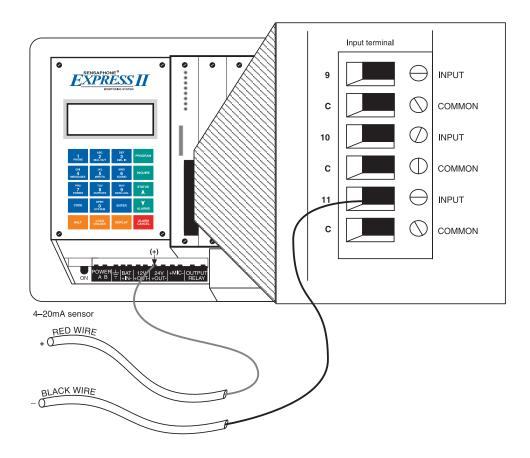
Figure 6: 4–20mA transducer using internal power supply
