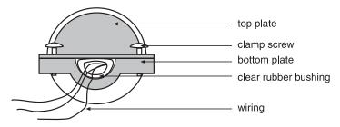
Figure 13: Strain relief clamp
