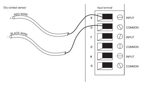
Figure 5: Dry contact sensor
