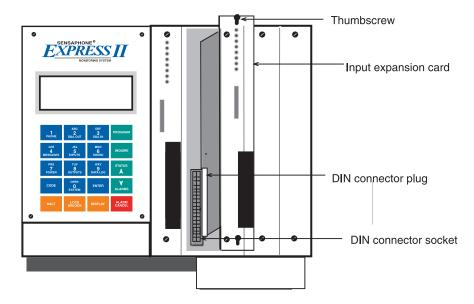
Figure 11: Line up and insert card
